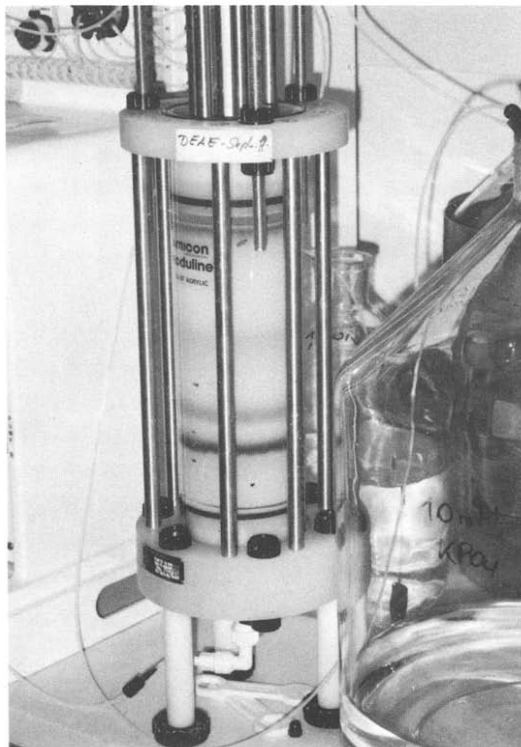
Fig. 9. Purification of SOD on the laboratory scale (18 cm \times 2.6 cm I.D. and 18 cm \times 9 cm I.D.). The small column was connected to an FPLC set-up and the large column to a Biopilot. A linear flow-rate of 25 cm/h was kept constant. The runs were carried out simultaneously with the same starting material. Identical patterns on the columns were observed.
